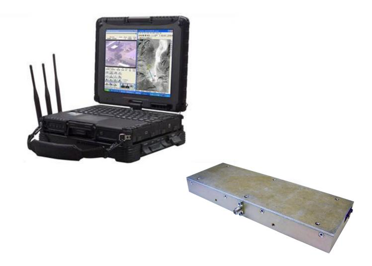
The LIDL Receiver is a four band receiver, operating in the L, S, low C, and high C bands. The LIDL is capable of operating in four unique modes supporting analog video with a tunable subcarrier, the Predator B waveform, the Plug and Play II waveform and a 70 MHz IF output. Other packages are available.
